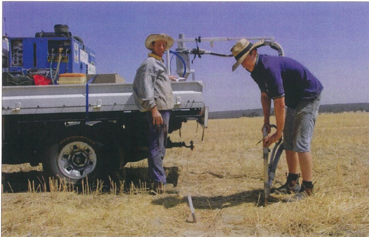
Figure 4 Soil sampling at Kellerberrin. Professional soil-sampling contractors should be able to accurately sample the soil profile.
